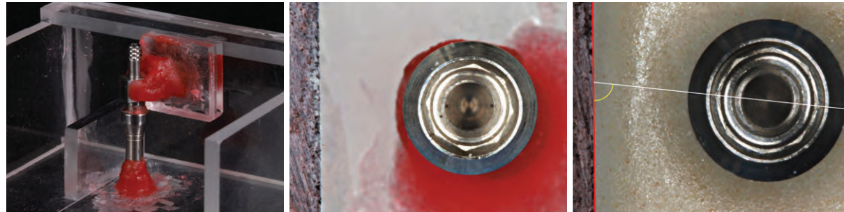
Fig. 3. A) Embedded fixture by resin, B) Set transpositional zig to base plate 1, C) Tightening IC and connecting IC to transpositional zig, D) Separating transpositional zig from base plate 1, connecting analog to IC and set to base plate 2, E) Image of analog, F) Measuring rotational error.
